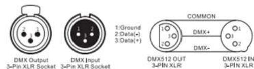
For installations where the DMX cable has to run a long distance or is in an electrically noisy environment, such as in a discotheque, it is recommended to use a DMX terminator. This helps in preventing corruption of the digital control signal by electrical noise. The DMX terminator is simply an XLR plug with a 120 Ω resistor connected between pins 2 and 3, which is then plugged into the output XLR socket of the last fixture in the chain. Please see illustrations
